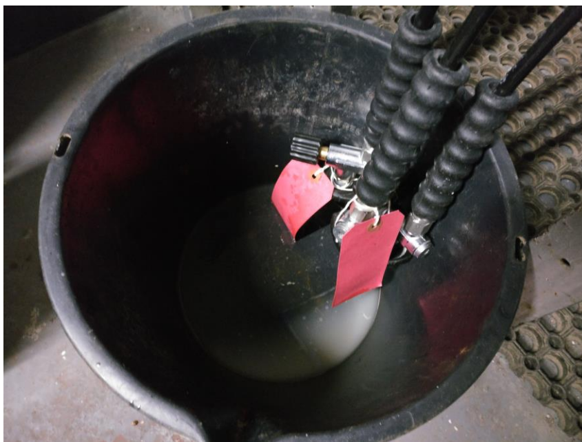
Figure 5 - A bucket catching the drips from the filling whips
