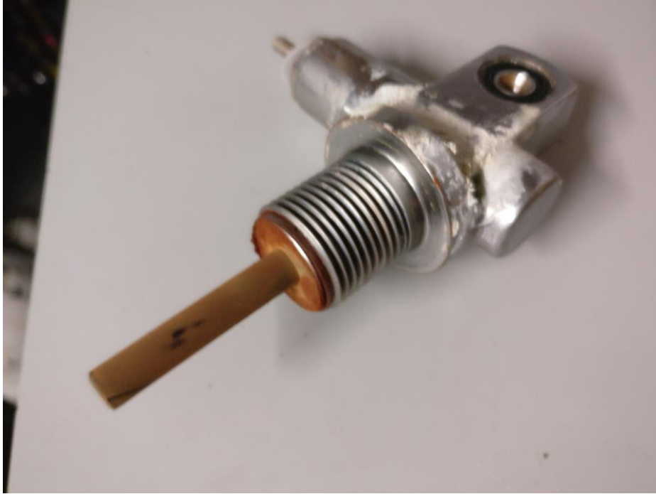
Figure 6 - The inside of the valve from the cylinder on which the issue occurred
