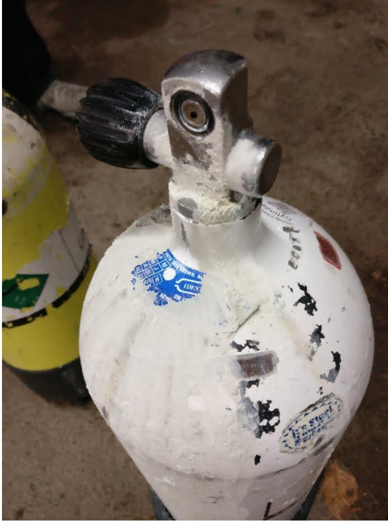
Figure 3 - The cylinder on which the O-ring failed. Note that it was in the DIN to A-clamp adaptor that the O-ring failed
