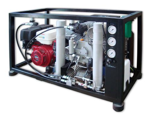
The charging times calculated below has assumed 12 litre water capacity cylinders with a working pressure of 232 bar, it has also been assumed that a residual pressure of 30 bar remains in each cylinder.
